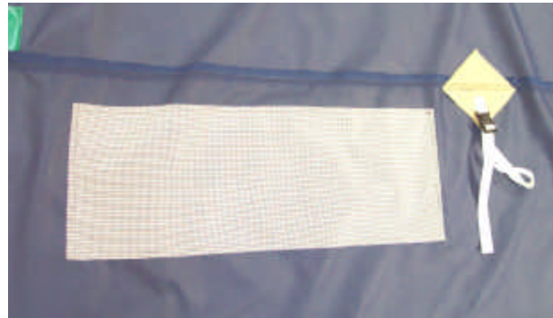
Tiedown and Ventilation screen detail
